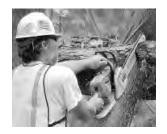
for the first time. Note especially how to check and adjust chain tension, which is vital for safe operation. Get more information about specific operations from a saw dealer, a book or video or from an experienced operator.
